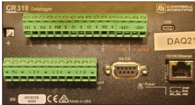
Figure 4.10: CR310 Datalogger by Maguire Mulligan.
